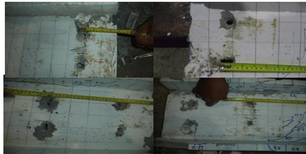
Gambar 4.10. Kerusakan lubang baut profil canal (c) ferro foam concrete
