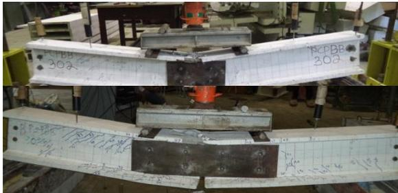
Gambar 4.8. Pola retak profil canal (c) ferro foam concrete
