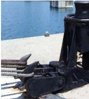
**Gambar 5. Double Mooring Quick Release Hook di Terminal Arun**
