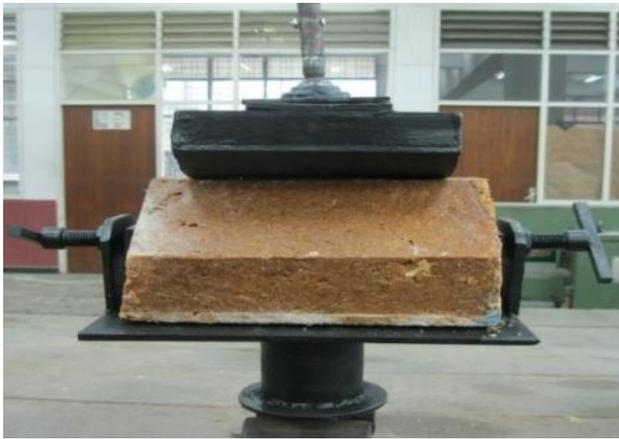
Gambar 23. Posisi anvil, parking bumper dan test rig
